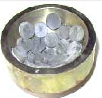
Curved pellet Plate To generate Spherically Ground Surfaces.
